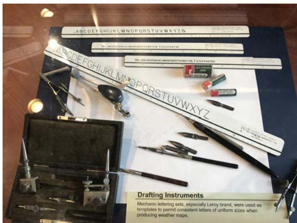
(Display) Drafting Instruments-Mechanical lettering sets were used as templates to permit consistent letters of uniform sizes.
